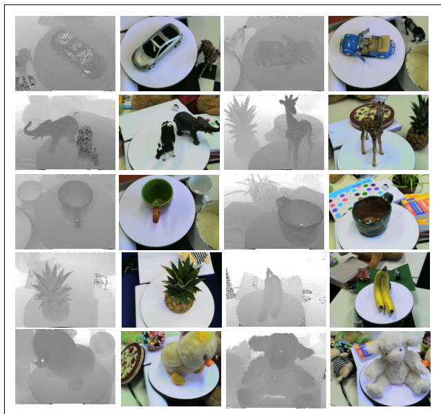
Figure 5.11: Example range images (using TOF PMD camera) and their corresponding color images (using CCD camera) of the JenaRange02 dataset. TOF PMD cameras produce reflected images with respect to images produced by CCD cameras.
