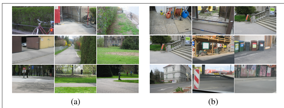
Figure 4.8: Example of incorrectly classified images on the Caltech dataset using the GLOH-color combination (GC-G). (a) Example of false negative images classified as background from the classes bikes (first row), cars (second row) and persons (third row). (b) Example of false positive images classified as bikes (first row), cars (second row) and persons (third row).
