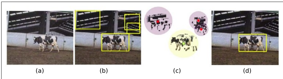
Figure 3.4: Stages of the model of Fritz et al. [52]. (a) Original images. (b) Generative part: hypotheses detected by the representative Implicit Shape Model (ISM) [80]. (c) Discriminative part: input to SVM stage. (d) Verified hypotheses.
