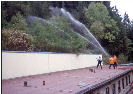
Figure 3.3: First hydrological experiment on 99/09/29: Firemen irrigate the roof area of the observatory (Kroner, 2002).
