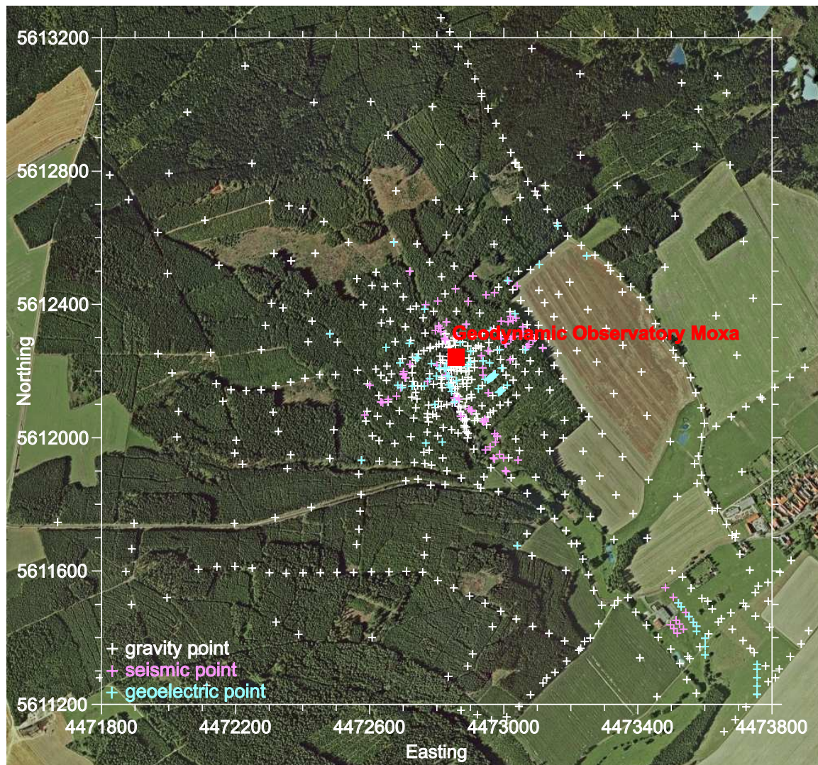
Figure 4.1: Gravimetric sites in the surroundings of Moxa observatory. The locations of geoelectrical soundings and seismic lines, which are used as constraints for the gravimetric model, are also given. The aerial photograph was taken from Google Earth (2008) .
