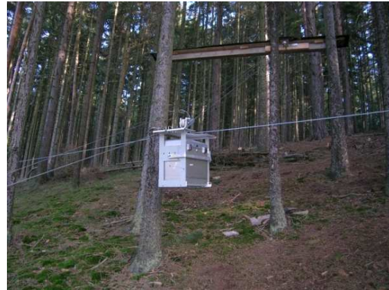
Figure 3.14: Gravimeter lift: upper station on the hill east of the observatory close to the point ET of the MoxaNet.
